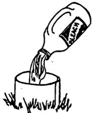
7. Close all valves and pour another 2 gallons of bleach directly into the well. Recap the well or replace the vent pipe or plug. Leave all valves closed for a period of 24 hours or longer.
